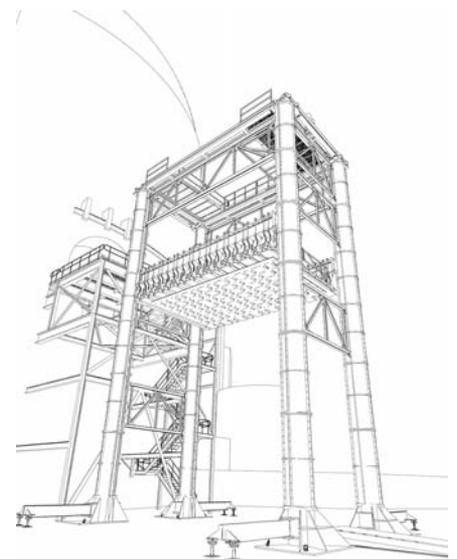
**The original design concept and the real-world result of the PMLS which was utilized at a nuclear power plant located in the Midwest to lift materials and equipment 50 feet above the ground to gain access to the building's only equipment hatch.**
