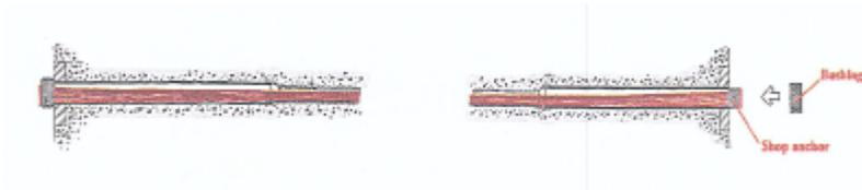
5. The tendon is ready for stressing. Depending on design considerations, tendons are stressed either at both ends or at one end only. The anchors at both ends accepted the identical stressing jack.
