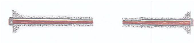
6. A hydraulic jack was coupled to the anchor to be stressed and exerted equal pull on the wires which are held securely in the anchor by their button-heads. As the tendon elongated and the anchor is pulled away from the bearing plate, steel shims of varying thicknesses, are inserted. When the required tendon elongation has been attained, the anchor is brought to rest on the shim stack.
