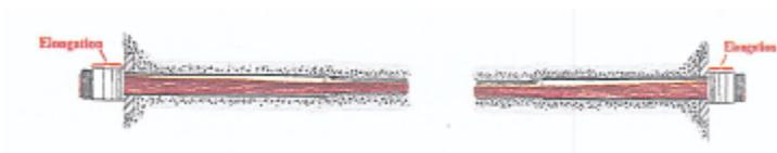
8. Grease caps with gaskets are positioned over the anchors at each end, and grease is pumped into the grease cap and through the conduit under pressure, completely encasing the tendon and its anchors for permanent corrosion protection.
